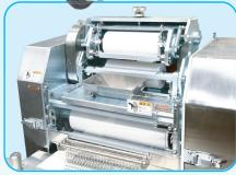
Upper roller section is able to tilt for easy cleaning,maintenance and sanitary. Only lower roller can be used with removal hopper(optional)
