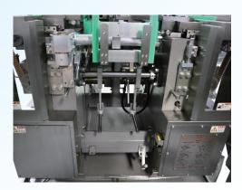
Dough chamber perfectly separated from driving section.
