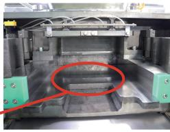
Front & bottom wear strips of dough chamber (i.e. sliding part) are easily replaced. Division head does not come in contact with sliding parts.
