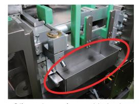
Oil catch pan located in both machine front and rear.
