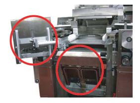
**Equipp**ed with cleaning aid device for main ram and knife. Even flip side easily cleaned.
