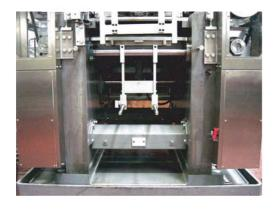
Dough chamber perfectly separated from driving section.
